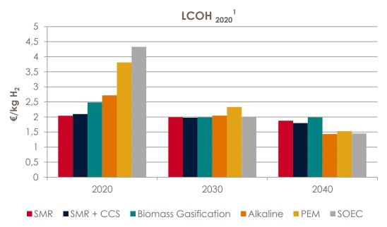
SMR (Steam Methane Reforming); SMR+CCS (Steam Methane Reforming with CO<sub>2</sub> capture; PEM electrolysis ( Polymeric electrocytic membrane); SOEC electrolysis ( Solide Oxide Electrolyzer)
