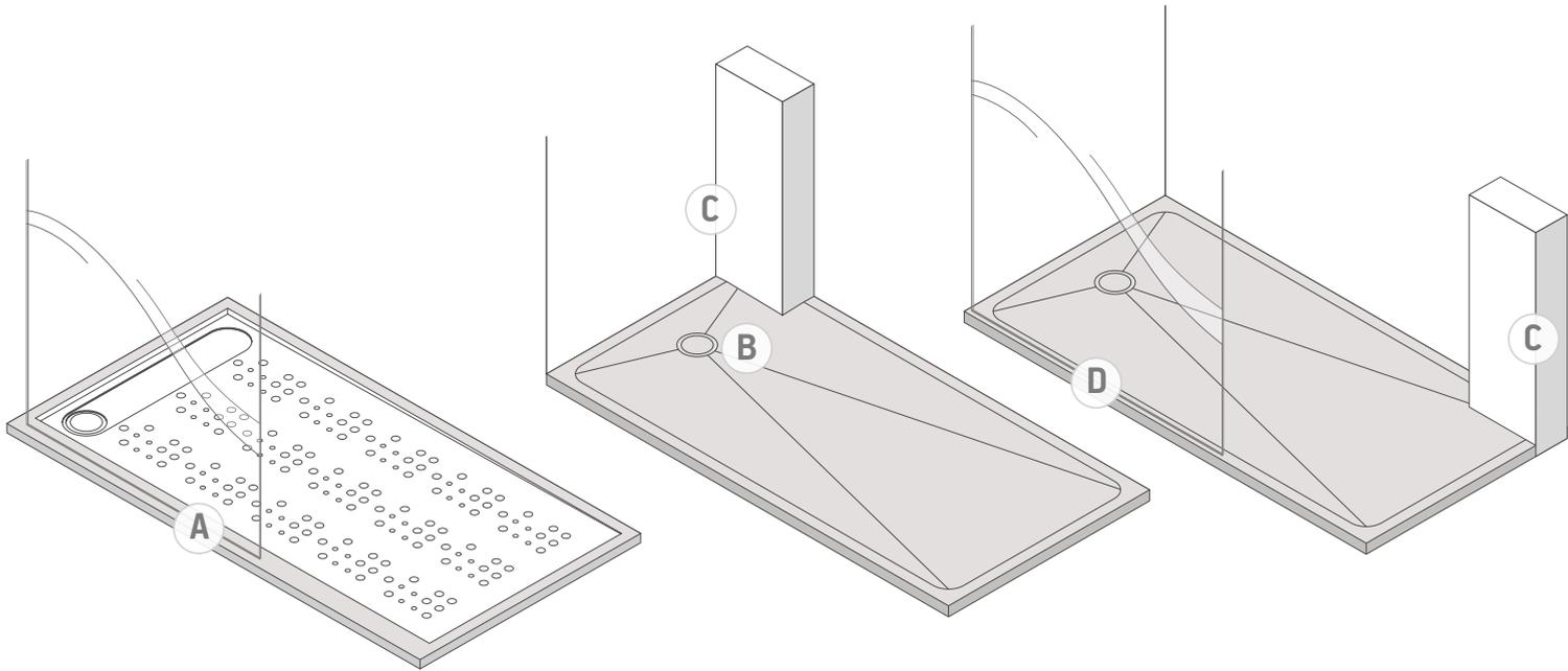
**A** Perimeter frame with a width of 4cm for supporting the screen
