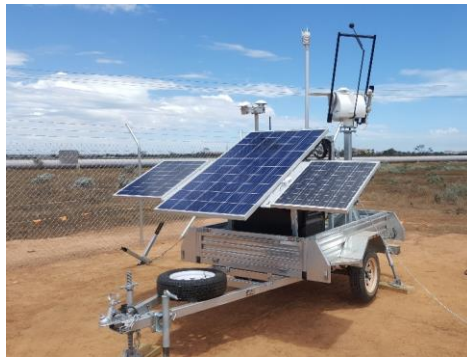
Fulcrum3D Met Station - solar monitoring
