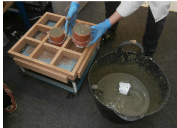
Figure 4: A photograph of the vibrating table used to remove air bubbles from the bentonite/ slurry mix.
