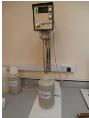
Figure 1: Photograph of the Silverson L4RT homogeniser used to thoroughly mix the separate slurry and binder mixes.
