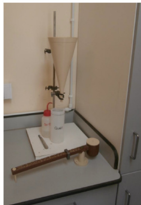
Figure 2: A photograph of the mud balance and density marsh cone viscosity tests which ensure the consistent quality of testing materials.
