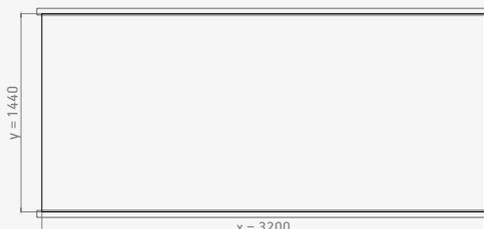
H1. Max. Design wind load: 0.5 kN/m<sup>2</sup>
