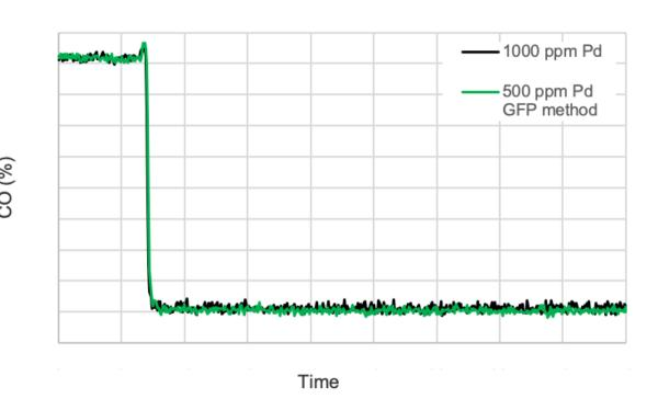
Data collected at CPERI indicated equivalent CO oxidation for ½ Pd content when promoter prepared using GFP method
