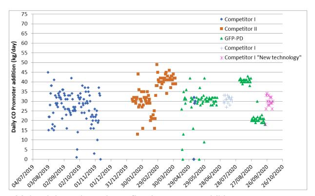
Main trial conducted at a fixed promoter addition rate at 30 kg/day for comparison. Other setpoints tested for sensitivity
