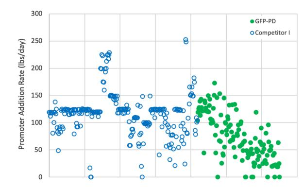
CO promoter addition rate controlled to achieve constant regenerator flue gas temperature
